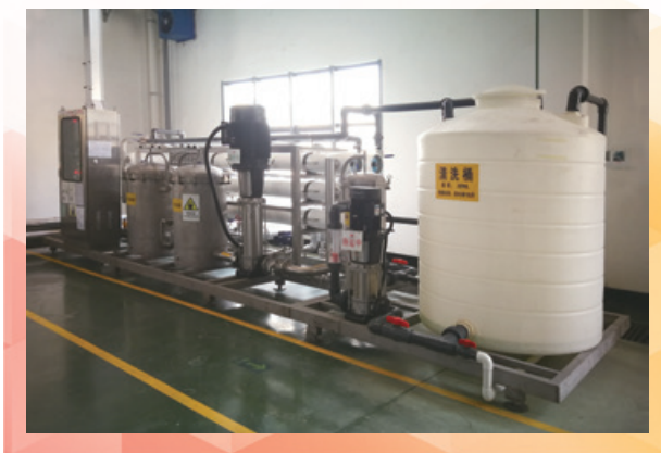
河南工廠反滲透濃水回收利用 Recycling of reverse osmosis concentrated water in Henan factory
